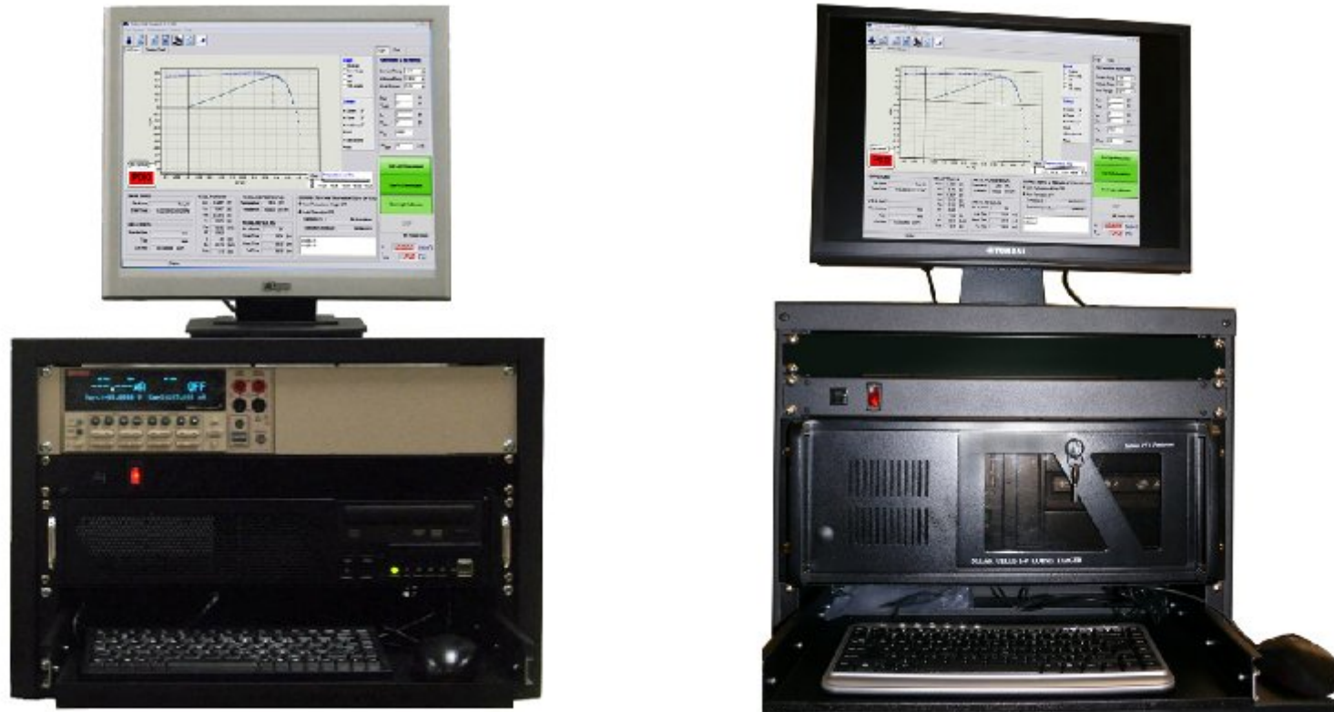
Figure 2: View of a Typical I-V System Console (Left view Model #'s CC1/CC3/CC5 : Right View Model #'s CC10/CC15/CC20)
