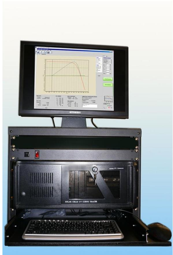
Figure 3: Typical I-V System Console – 15A/20A Current
