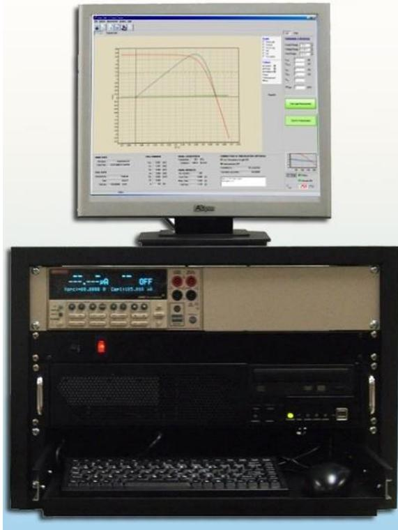
Figure 2: Typical I-V System Console -  $\leq 5A$  Current
