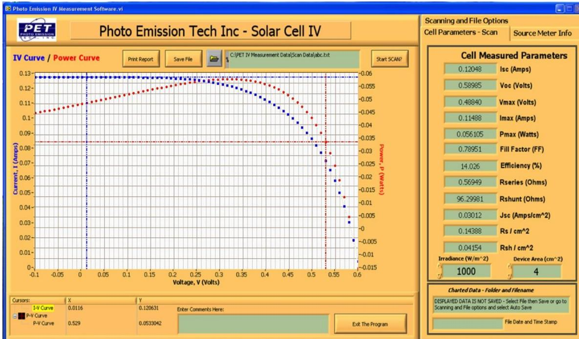
Figure 4: Cell Parameter Scan Screen
