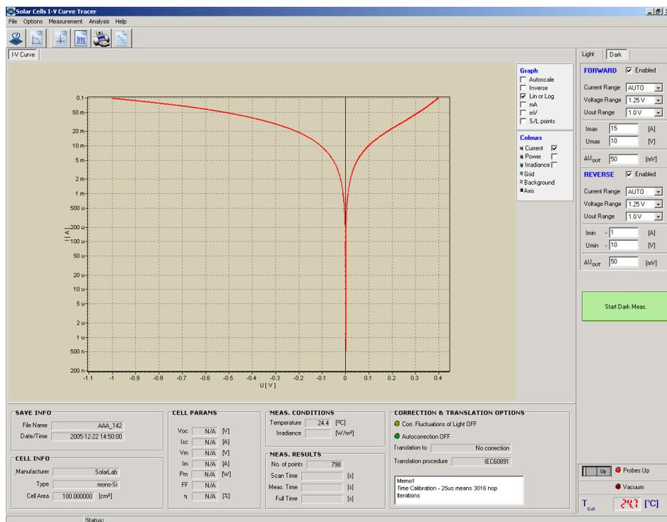
Figure 8 : Example of “dark” measurement – Advance Software
