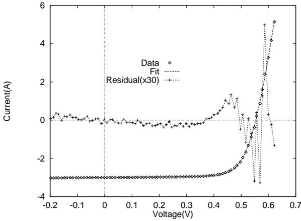
Fig. 1: Unweighted least squares fit to an I-V curve. The data points have been calculated with  $I_{01} = 1. \times 10^{-9}A$ ,  $I_{02} = 2. \times 10^{-5}A$ ,  $G_{sh} = .1S$ ,  $R_{se} = 7m\Omega$ ,  $I_{lt} = -3A$ . A voltage noise of 1mV and a current noise of 3mA was added.
