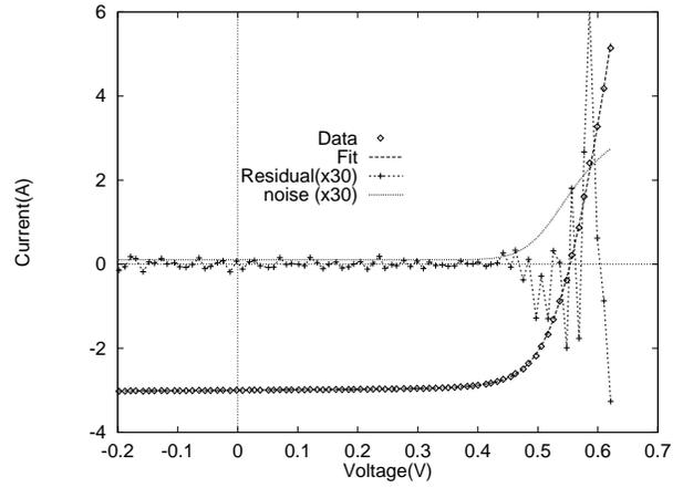
Fig. 4: Weighted least squares fit to the same data as in Fig. 1. The curve marked "Noise" refers to the total noise level from equation (6)
