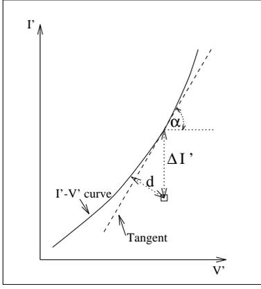
Fig. 3: An approximate value for the distance of a measured point ( $\square$ ) to the fitted noise scaled I-V curve (solid line) can be obtained from the current residual  $\Delta I'$  at that point and the slope  $\alpha$  of the curve
