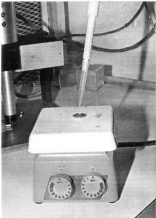
To begin the measurement, a clean cup is placed under the probe of the SQM 200. A guide is used to ensure repeatable positioning. A reading on the SQM 200 is taken after allowing 10 seconds for the signal to stabilize. A minimum photocurrent reading for the clean cup must be achieved; otherwise, the cup is set aside for recleaning and another clean cup is selected.
