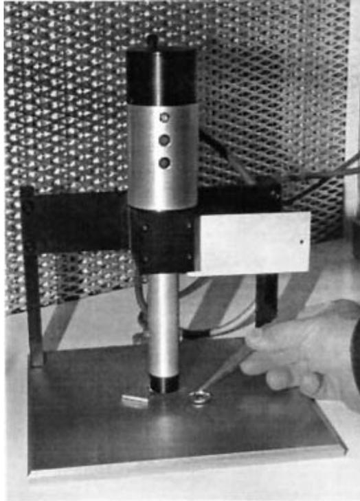
After the cup has cooled, it is replaced under the probe and a reading taken in the same manner as previously described. The dosing, evaporation, cooling, and measurement steps may be repeated up to five times to build up any contaminants present in the solvent to obtain the required confidence in the cleanliness measurements.
